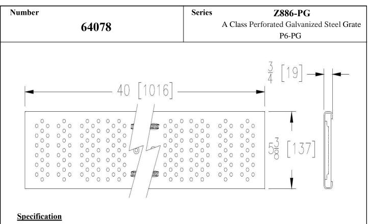
The Zurn P6-PG Fabricated Perforated, Galvanized Steel Grate, is 5-3/8 inches wide by 40 inches long, weighing 1.6 lbs per linear foot. The grate has an open area of 5.3 square inches per linear foot, DIN Rating of A, ANSI Rating of Light Duty, ADA Compliant. Galvanizing conforms to ASTM specification A653, Galvanized Coating designation G60, minimum spangle. Supplied by Trench Drain Supply.
